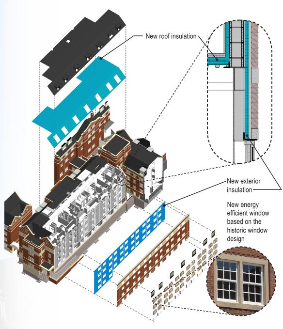
The existing building envelope was reused and brought above code requirements through the use of current construction techniques and materials, including thermal imaging. Thermal imaging was used to detect areas of heat loss in the existing building envelope. These
